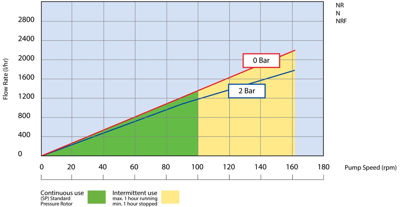
Flows are typical and were measured with water at 20°C with no suction lift or discharge pressure. Actual flows will vary according to suction conditions, discharge pressure and normal component production tolerances.
