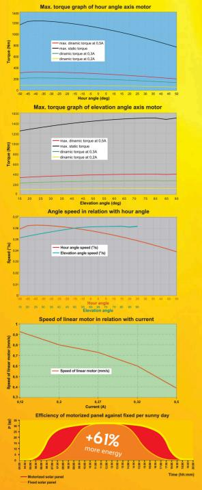
Real energy measurement of two equal solar panels (fixed and motorized)
