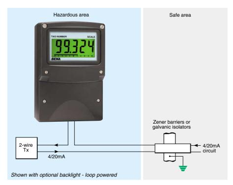
The BA324E loop powered 4/20mA indicator is a fourth generation field mounting instrument that is electrically and mechanically compatible with the earlier BA324D. It has a much larger full 5 digit display and guaranteed performance between -40 and +70°C. Like it's predecessor, the BA324E is housed in a robust IP66 enclosure with a separate terminal compartment.
