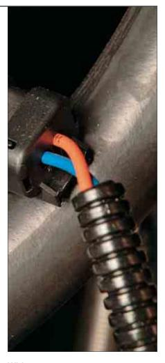
Wiring. With heavy-duty wiring, Cat Compact Wheel Loaders offer great electrical durability. The water resistant sealed connectors prevent dust and moisture interfering with the electrics. Multicoloured wiring is used to ease diagnosis and fault finding.
