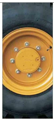
**Heavy Duty Axles.** The H Series Compact Wheel Loaders are fitted with heavy duty axles, with outboard planetary reduction gears.
