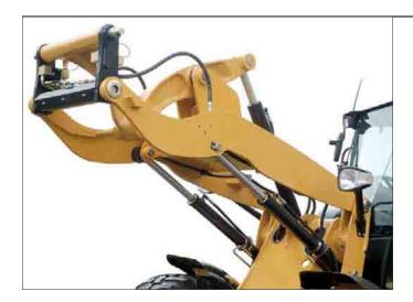
**Z-Bar Design.** Each of the Caterpillar Compact Wheel Loaders make use of the high performance Z-bar loader design which has been optimized for strength, visibility and versatile attachment usage.
