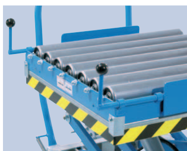
| Roller conveyor with hand released, gravity operated stoppers
