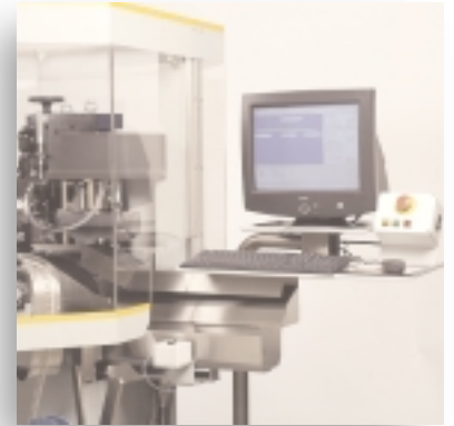
An ergonomically designed PC workstation has been built right into STX wire processors.
