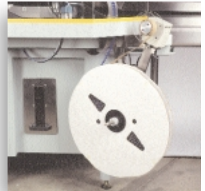
Terminal reels are loaded below the working platform on the STX to minimize lifting during a changeover. Paper take-up devices are also available for collection of terminal reel paper waste.
