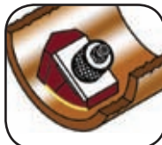
Circumferential Inside Diameter
