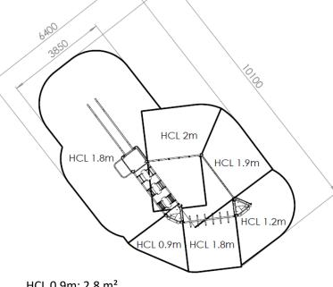
HCL 0.9m: 2.8 m<sup>2</sup> HCL 1.2m: 5.2 m<sup>2</sup> HCL 1.8m: 25.4 m<sup>2</sup> HCL 1.9m: 6.4 m<sup>2</sup> HCL 2m: 8.7 m<sup>2</sup> Surface totale: 48.5 m<sup>2</sup>
