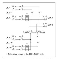
Scanner Configuration for Models 2000-SCAN and 2001-SCAN
