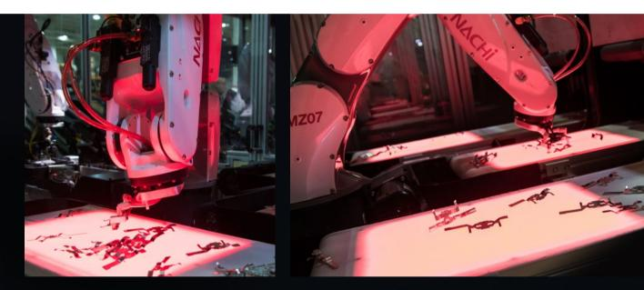
Pick-and-place robot application in which a very bright custom back light shines through the conveyor belt and thus enables machine vision for the robot.
