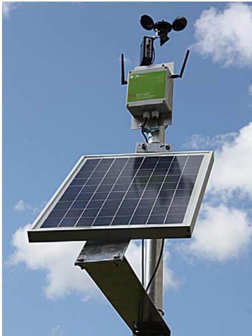
Utilising GPRS network to output data from T24 inputs to servers, email address and mobile phones
