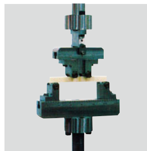
Three-/four-point bending test jig for plastics
