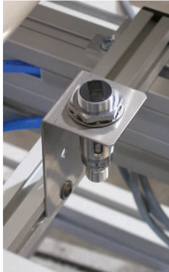
Initiator holder made from VA steel sheet
