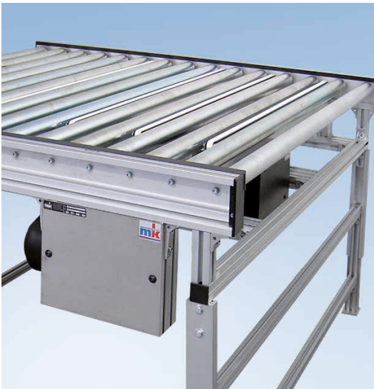
Tangential chain roller conveyor RBT-P 2255 with ø 50 mm steel rollers and tangential chain drive
