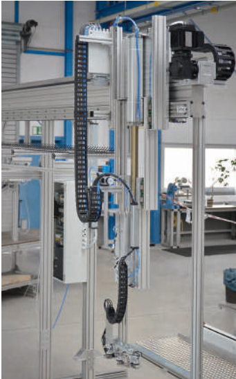
Gantry stand with telescopic gripper unit
