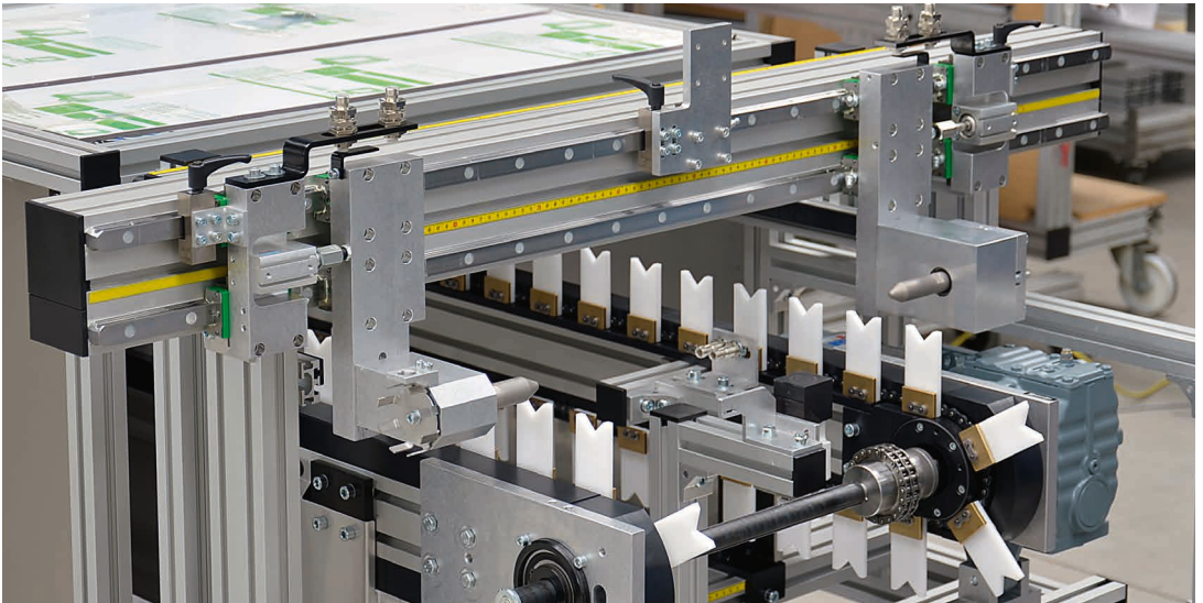
Timing chain conveyor with alignment unit for camshafts using recirculating ball bearing guide
