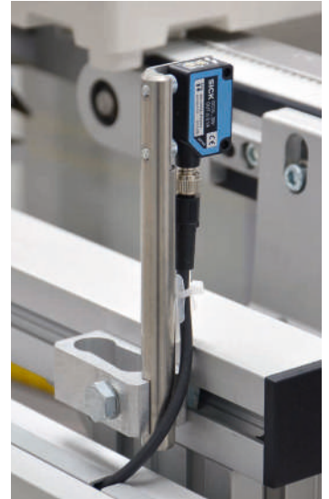
Photoelectric sensor with adjustable holder
