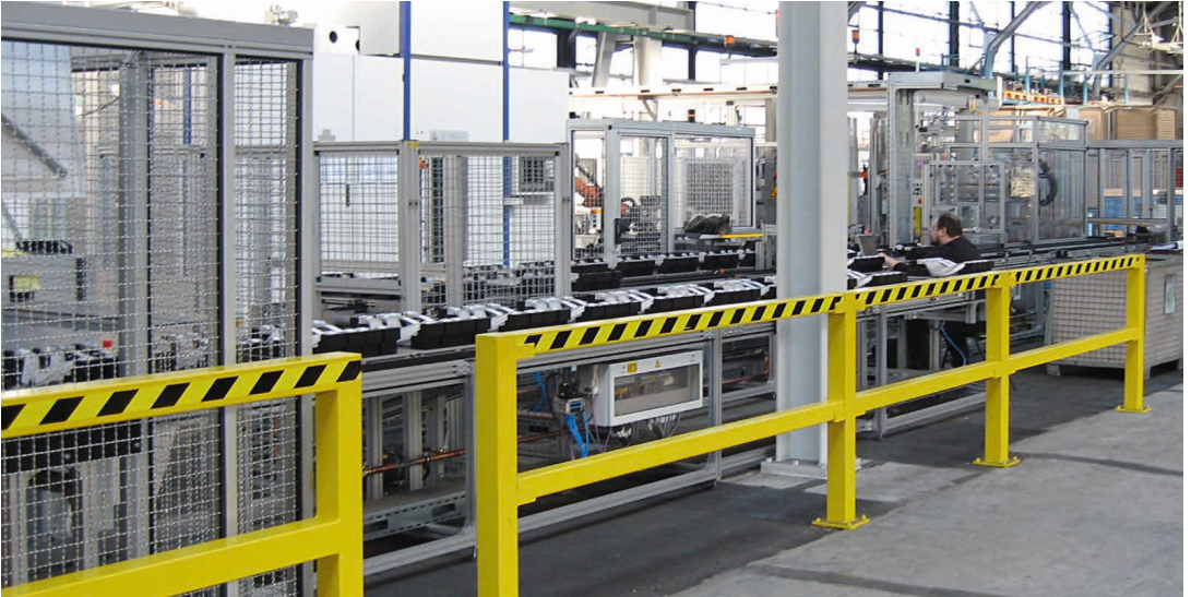
Interlinking production cells in the automotive industry Manual pallet stocking, removal with customer-supplied handling system and robot. Lower return level with lift and shuttle.
