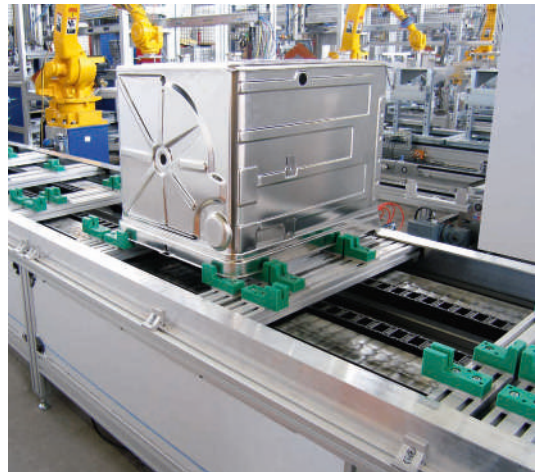
SPU double-line as an infeed conveyor for dishwasher housings
