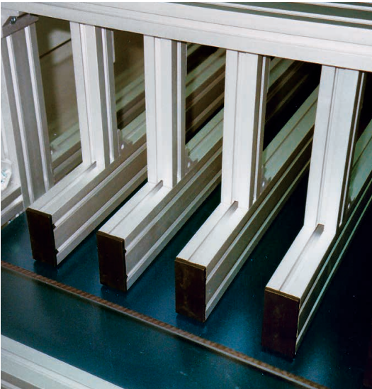
Multi-line, adjustable side rail in gantry arrangement
