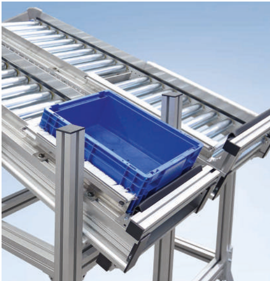
Gravity roller conveyor RBS-P 2255 with angled VA sheet steel as side rail, brush strip and end stop at the conveyor outfeed
