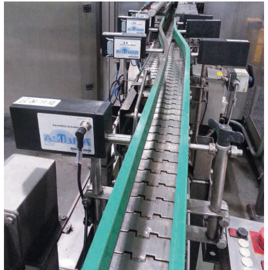
Versaflex SBF stainless steel conveyor with automatically adjustable side rail ASTRRA
