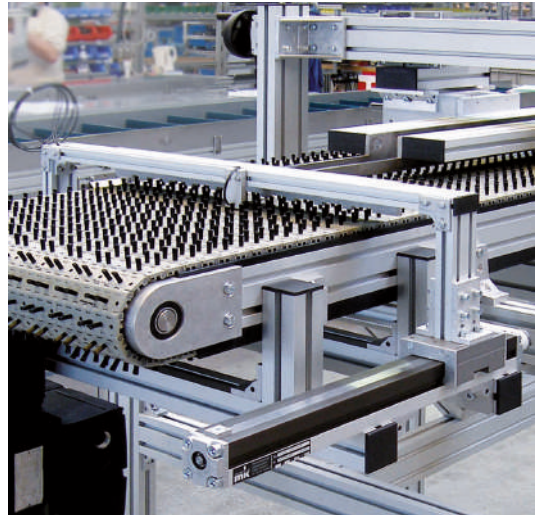
Modular belt conveyor MBF-P 2040 with head drive AC and plastic bristles for gentle transport
