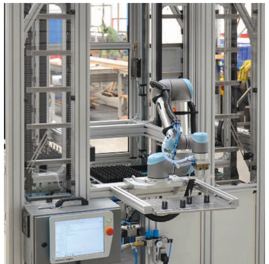
Production cell with paternoster storage for infed and discharged parts
