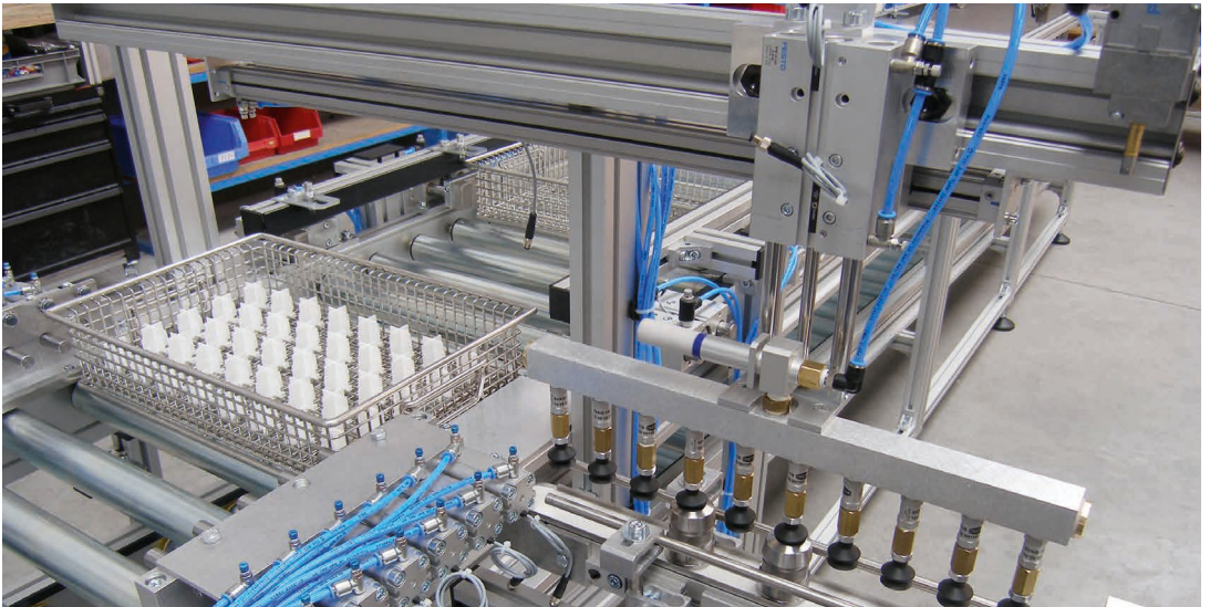
Pneumatic linear module with PF 38.77 and LW 38.77-44 as a transfer unit with 10 vacuum suction grippers
