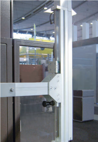
Electromotive VST 2015 with recirculating ball bearing guide
