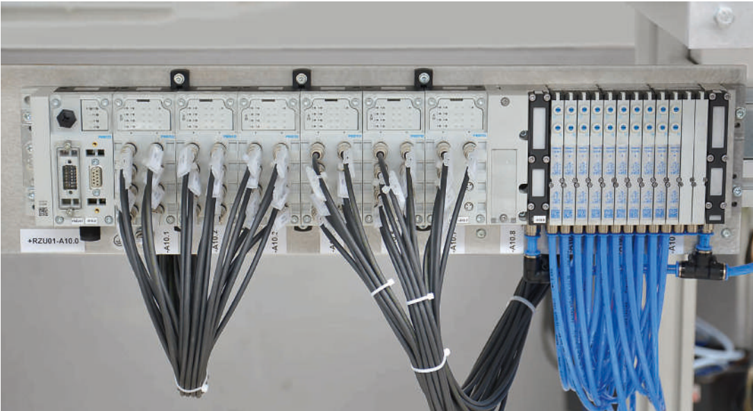
Valve terminal with input and output module
