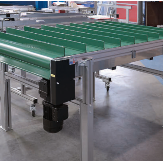
GUF-P 2041, head drive AC with support pan and transverse cleats
