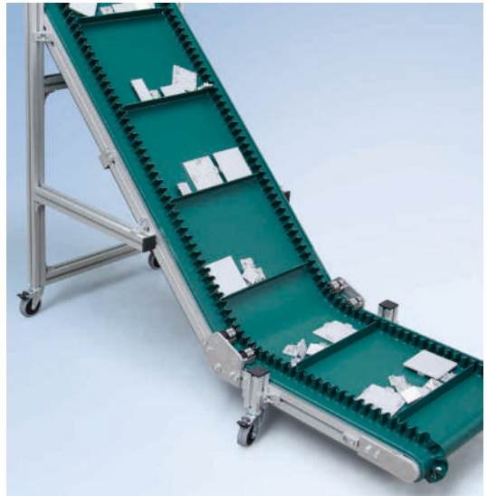
Incline conveyor belt KFG-P 2000 ECO with 45° incline, option B2 (B20.00.015-B2)
