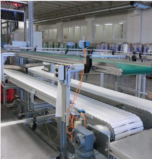
Versaflex flat top chain conveyor as clamping conveyor
