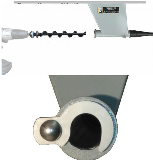
Engage the endless screw in the tank, and then turn the screw lock.
