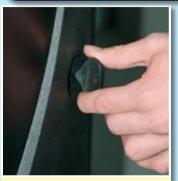
1. Insert the key into the lock and unlock clockwise.
