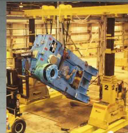
Boom strength easily allows two leg press tip up
