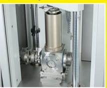
Volumetric dosing of HDP – high accuracy of filling quantity
