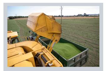
The tipping height of the large capacity pea hopper is variable from 2.9 to 3.4 metres making the 1089 easy to use with a wide range of trailers or high-sided containers.
