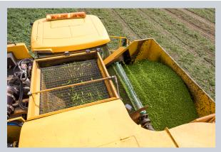
The 1089 utilises the latest design of Podder Chain. The stainless steel link-wire belt has outstanding reliability and requires only a minimal amount of maintenance.
