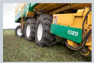
The four wheel steering makes the 1089 very manoeuvrable, increasing in field efficiency and reducing overall field damage.
