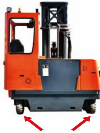
Dual drive, dual electromagnetic braking
