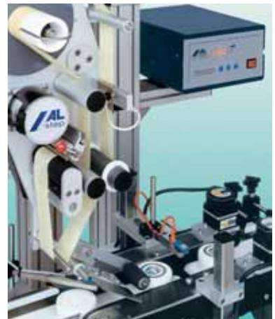
where cost reduction is a crucial requirement. The control panel makes it possible to adjust the main functioning parameters (speed and pre-dispensing) by means of digital indicators (contraves), emitting an end-of-roll or web-break alarm signal. A label sensor for transparent material is optionally available.
