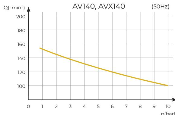
Compressor pump efficiency
