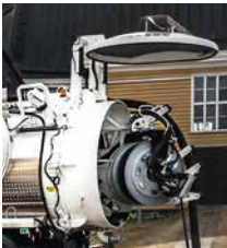
Covered hose reel
