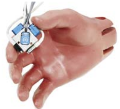
A six-axis package is easily obtained by taking the DTS ARS triax package and mounting three Endevco 7264 or MSI 64 accelerometers.
