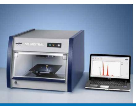
The M1 MISTRAL is a compact spectrometer for the analysis of bulk materials and layers using X-ray fluorescence technology. It allows non-destructive measurements on a wide range of sample sizes without the need for sample preparation.
