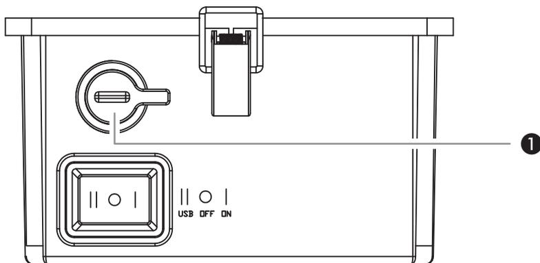
To switch the light on set the switch to the "I" (ON) position. To switch it off, set the switch to the middle position, "O" (OFF).
