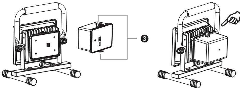
The battery is quick and easy to replace. Simply open the two fasteners 3 at the top and bottom, see drawing. This makes it possible, for instance, to charge the battery while continuing to work with the spare battery (if included) or the replacement battery (available separately).
