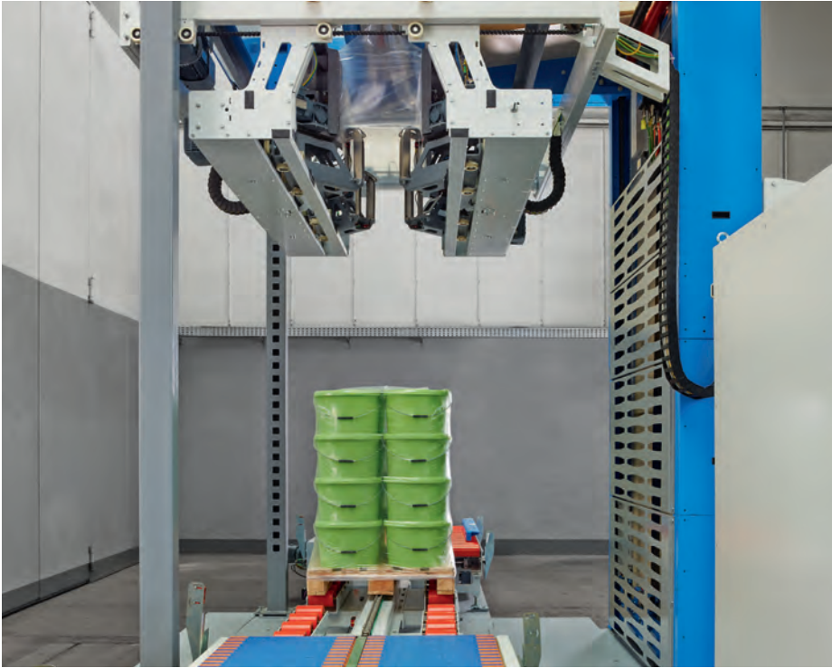
All types of packaged goods can be protected by a waterproof film hood.
