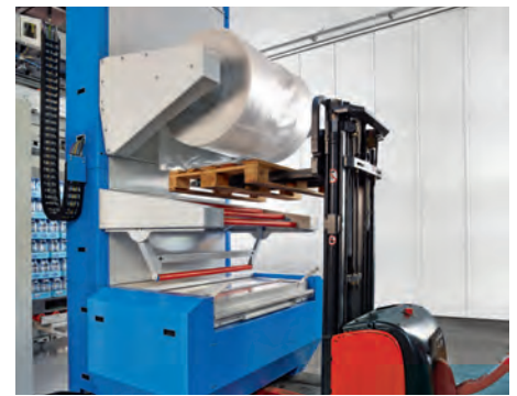
Positioning the film roll works with a few easy actions and without tools.
