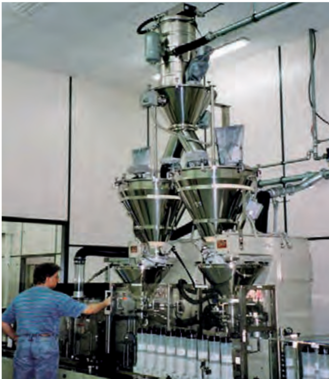
Loading a toner filling system.
