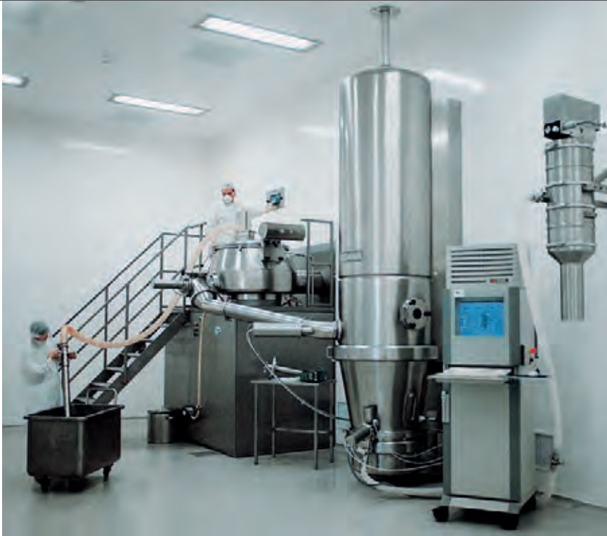
Vacuum conveyor for automatically emptying a fluidized bed dryer. Product is dispensed via an immersion pipe into IBCs.
