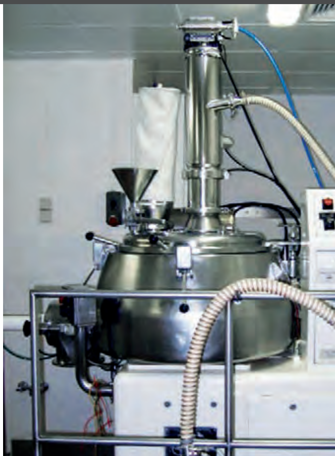
Loading of the mixer using PPC.
