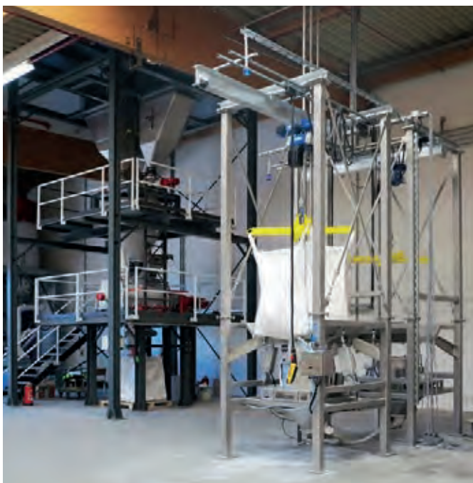
Big-Bag discharging station for conveying of various powders (some are abrasive) into a mixer.
