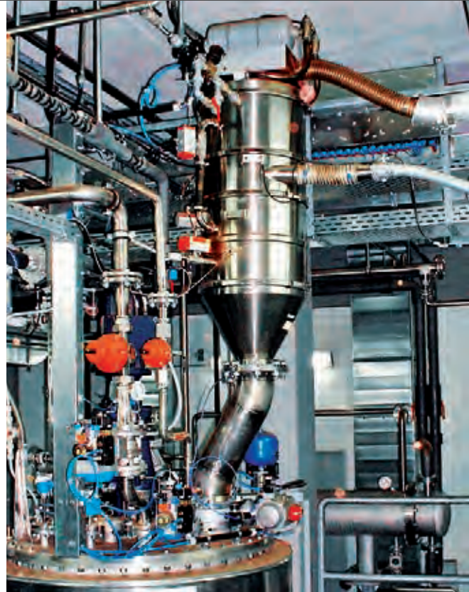
Vacuum conveyor with a powder lock for conveying pigments in a solvent atmosphere.
