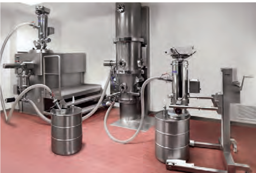
Emptying the drum and loading the mixer; Emptying a fluidized bed dryer and filling the drum.
