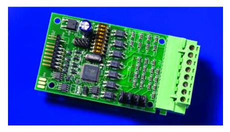
configurable as watchdog relays, group relays, horn relays, ring-back relay or diagnostic relays.
