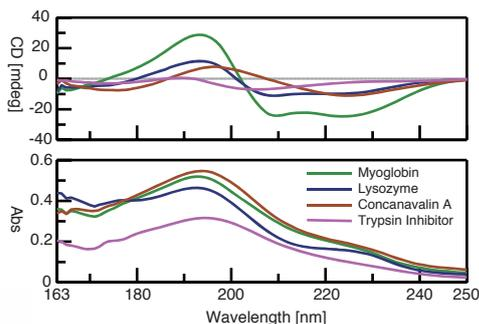
The innovative optical system of the J-1500 allows the measurement of a CD spectrum in the vacuum UV region down to 163 nm. The vacuum UV region below 200 nm, is of critical importance for biomolecules, particularly in protein secondary structure estimation. The data shows a CD and Abs spectra of various protein films, proving superior S/N ratio in the vacuum UV region below 170 nm.
