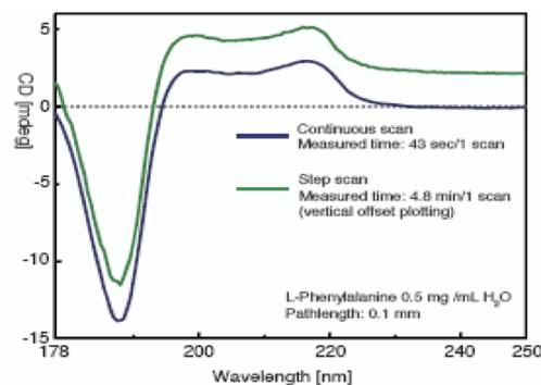
High sensitivity combined with a maximum of 10000 nm per minute scan speed allows the J-1500 to measure samples quickly increasing productivity in your lab. An additional benefit is the minimal time exposure of biological samples to the high-energy UV light minimizing the risk of sample degradation. The figure shows rapid spectral measurement of L-Phenylalanine solution measured with a data pitch of 0.1 nm. The measurement time was only 43 seconds per scan.
