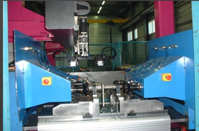
Extremities shaft machining
