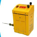
Provide mechanical excitation with speed adjustment to check transducer health
