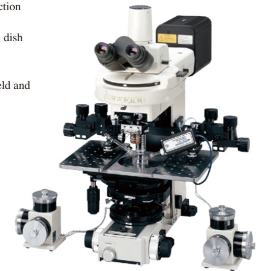
Configuration with Narishige micromanipulators and epi-fluorescence attachment
