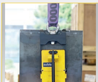
↳ Transport vertical Fv = 1/3 Fh
