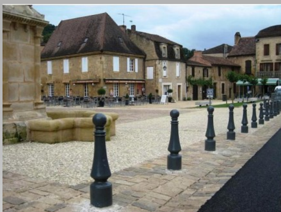
71 ARVERNUS-22 fonte d'acier, RAL, 3 hauteurs, scellement direct ou amovible | cast-iron post, 3 height options, RAL coated, to be concreted, or removable.
