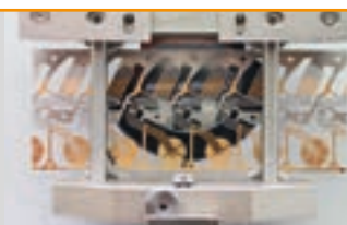
Sensor contacts: Au/Ni/CuFe
