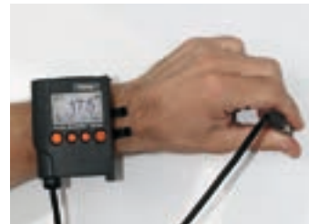
Wristband for MPOR-FP instruments for one-hand operation
