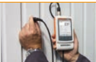
Measuring paint coating on steel
