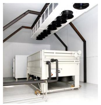
Unit under test in large calorimeter room
